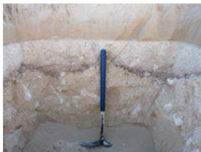
To the left: An excavated pit exposes an organic rich horizon and erosional disconformity within bioturbated carbonate-rich dune sand. The horizontal contact between the carbonate-rich sediment and modern dune sand is apparent at the top of the photo. Most „outcrop” in the field area was only accessible after a lot of digging. The pick, included for scale, is 60 cm long.
